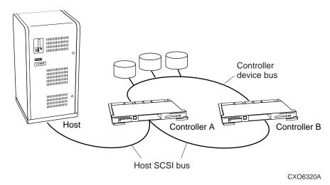
Figure 2–7. Host SCSI Bus and Controller Device Bus
